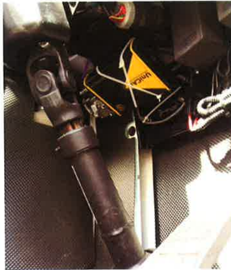
CAN data logger installed
