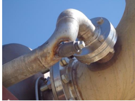
Figure 11: H 2 Injection Port for Strategy I
