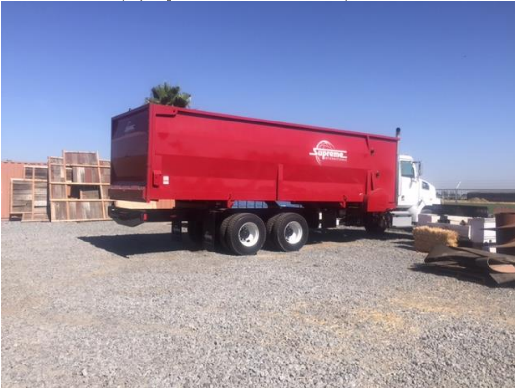
Picture 7: Assembly of Supreme International delivery box on Western Star truck
