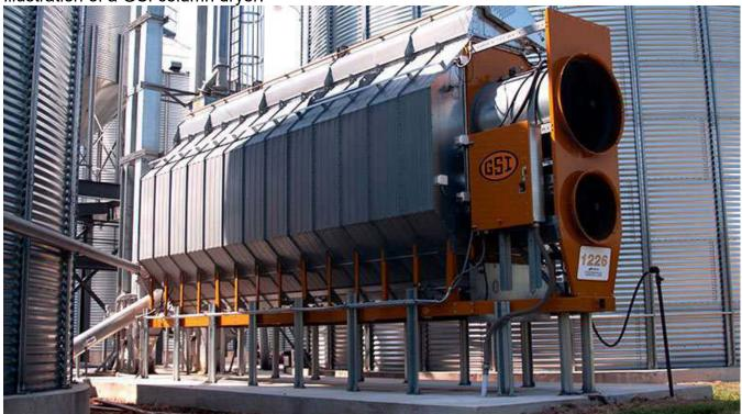
In this representative image of a GSI 1226X column dryer. Exhaust escapes through small perforations, which are too small to be seen in the photo, covering the sides and top of the column dryer.
