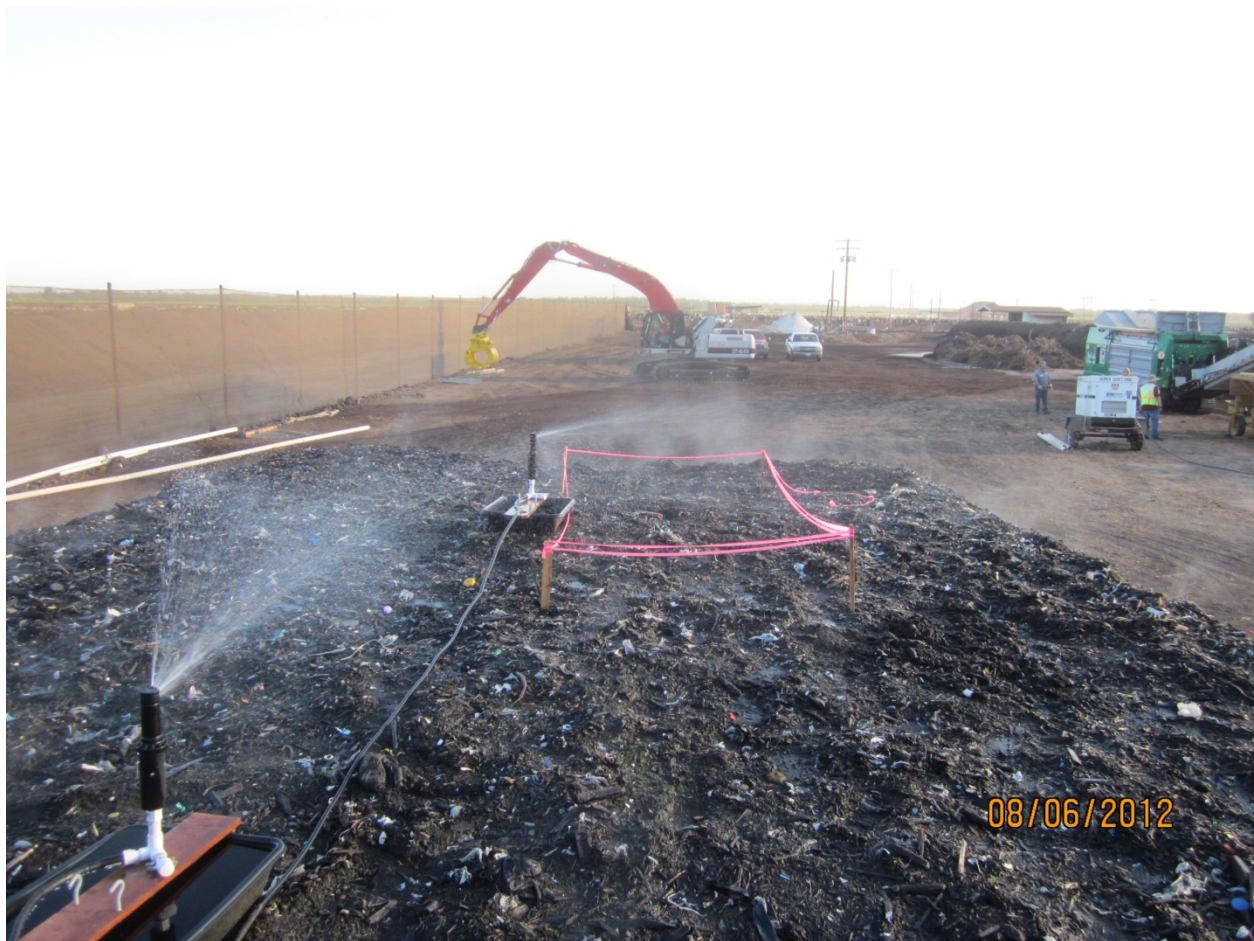
Photo 4: Irrigation sleds wetting top of prototype eASP. Note- test areas cordoned off for air emissions sampling.
