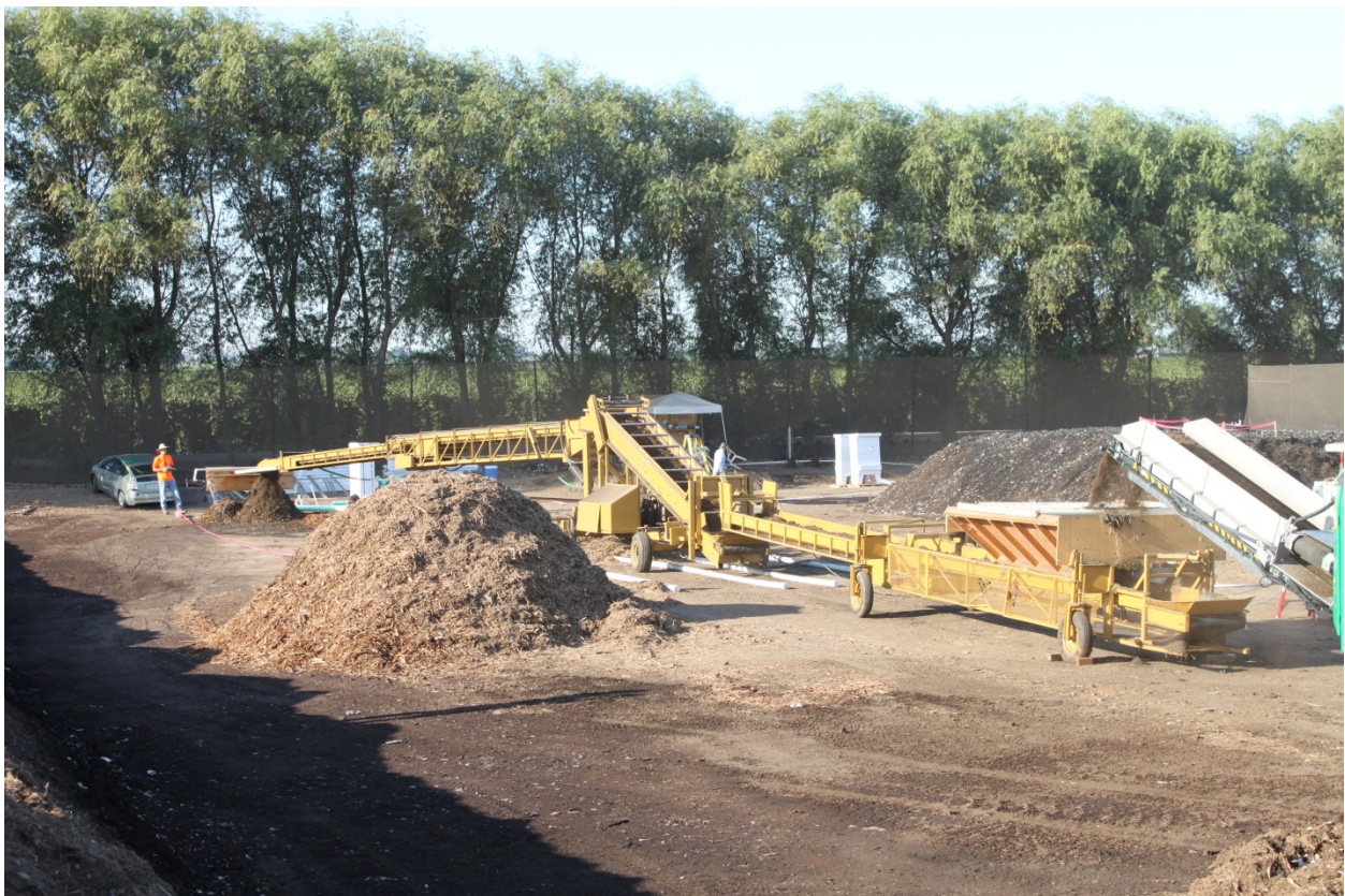
Photo 2: Complete conveyor train. Material discharged from the shredder, far right, falls into a specially constructed hopper on the intermediate conveyor, and then is deposited into the hopper of the potato piler, center. From here the materials are carried upward and across the potato piler before being discharged at the far left,
