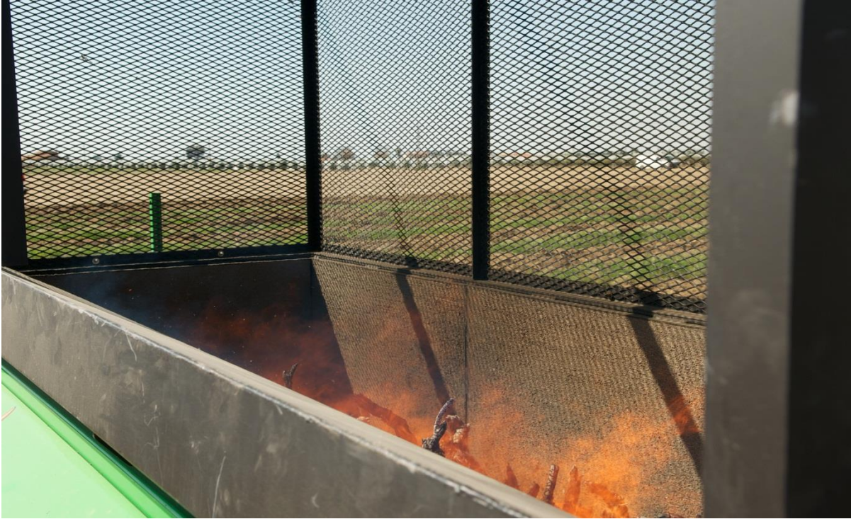
Fig. 2 Burn Boss® Air Curtain Burner with grape stumps
