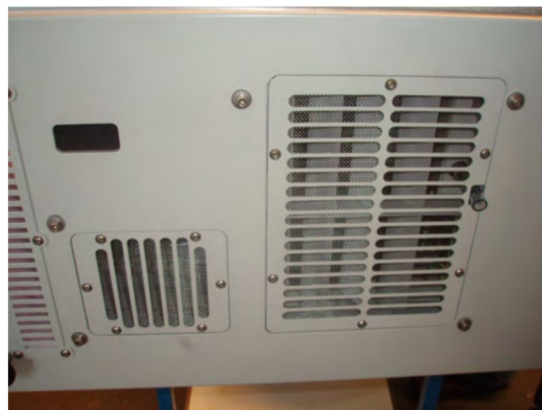
Figure 11.19.: Ventilation grids of the airpointer
