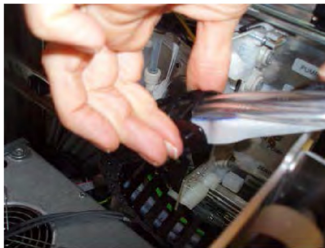
Figure 11.10.: Loose the clamp
