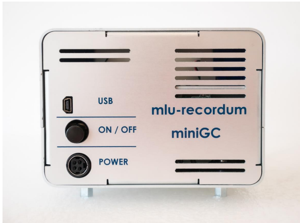
FIGURE 9: BACK VIEW OF THE BTEX-GC BENCH WITH ELECTRICAL CONNECTIONS
