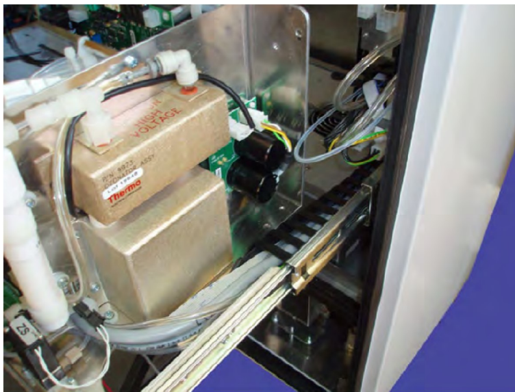
Figure 11.7.: Push and pull the module on both sides simultaneously
