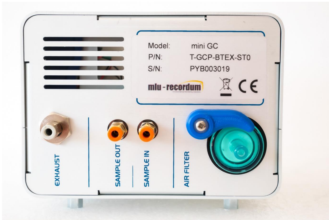
FIGURE 8: FRONT VIEW OF THE BTEX-GC BENCH WITH PNEUMATIC CONNECTIONS
