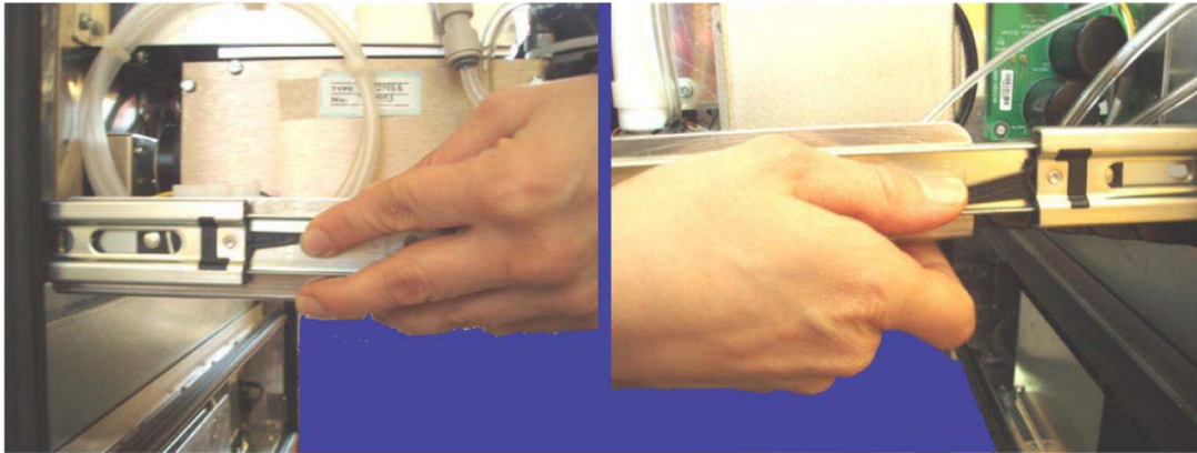
Figure 11.11.: Press the small levers in both drawers up (left) or down (right).
