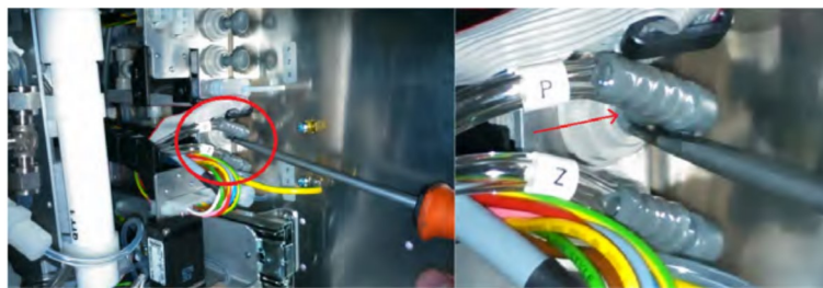
Figure 11.9.: Pushing down the grey ring with a screwdriver
