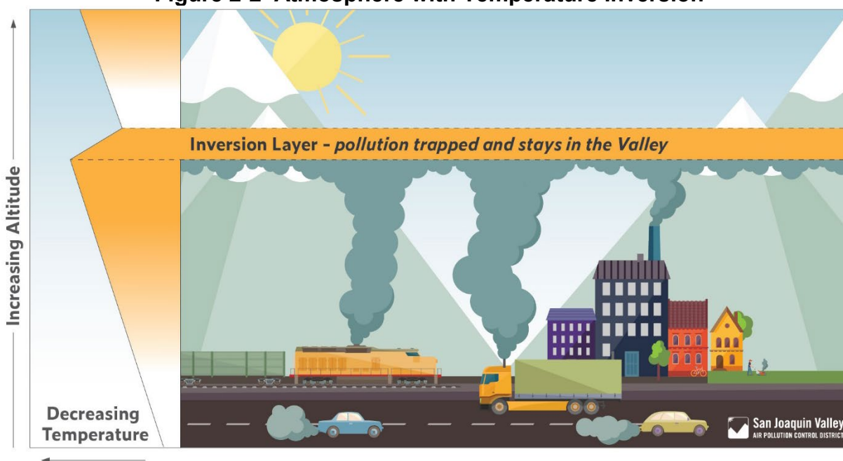
Figure 2-2 Atmosphere with Temperature Inversion
